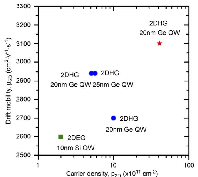
Fig. 1. The drift mobility as a function of carrier density at room temperature. The 2DHG in a 20 and 25 nm Ge QWs from Refs. [1,3–5] are shown by circles. The 2DHG in a 20 nm Ge QW obtained in this work is shown by star. The 2DEG in a 10 nm Si QW from Ref. [7] is shown by square.
